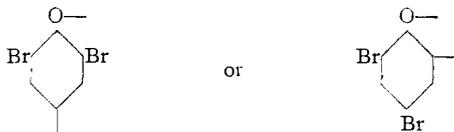
which then polymerize to a compound of high molecular weight,  $(C_6H_2Br_2O)_n$ , for which the name poly-dibromo-phenylene oxide has been suggested.<sup>3</sup>
